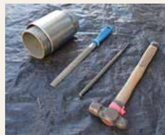
**Repair equipment.** Ball peen hammer, files, large metal cylinder.
