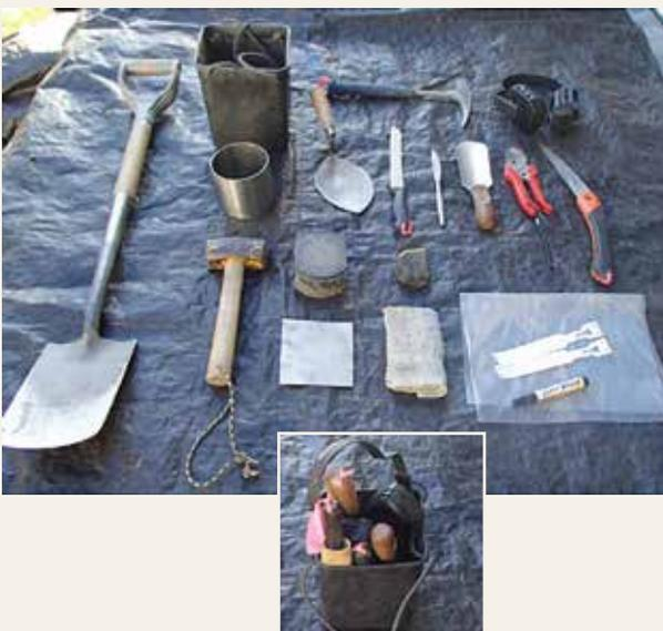
**Sampling equipment.** Spade, 10 cm soil cores (x2), peg hammer, spigot block, metal plate, flat trowel, cleaning cloth, cutting knife, table knife, trowel, pruning saw, secateurs, earmuffs, 3 m of retractable tape, geological hammer, 5 L bucket, kneeling pad (optional), soil bags, sample tags, Vivid marker pen.
