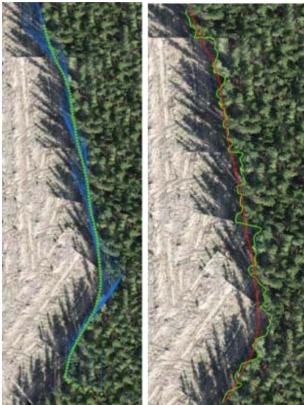
**Fig. 2.** Left panel shows the UAV flight path (dotted green) and heading (blue lines) determined by edge detection. Right panel shows the smoothed flight path (red) compared to the actual edge determined from ground-truth mapping (green).
