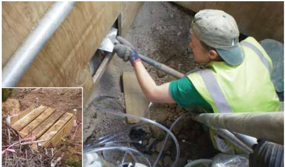
Amanda Matson installing lysimeters in a soil pit and completed pit directly after fertiliser application (inset).
