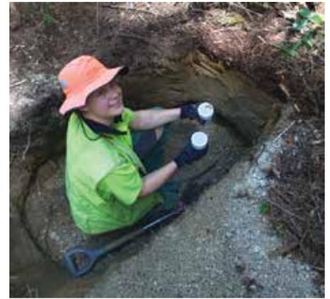
*Loretta Garrett installing resin lysimeters into a soil pit in the Timberlands biuret trial.*
