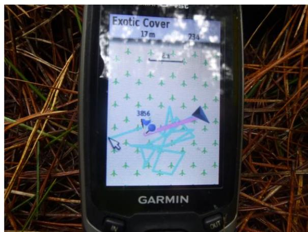
**Figure 4.** Random GNSS error when static (blue line).
